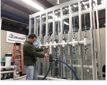
Test wall can accommodate products up to 2438 mm W. X 2438 mm H.
